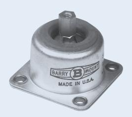
Barry S-Mounts are air-damped isolators and are designed to provide the highest degree of vibration isolation for sensitive commercial and military airborne equipment. S-Mounts are particularly effective at isolating low level vibration.
