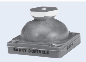
Barry HTTA-Series Mounts are low frequency isolators with a large deflection capacity to provide both vibration and shock protection. They are designed to meet the requirements of MIL-STD-810C for mounting electronic equipment in helicopter environments.
