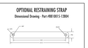
\*Please note, mounts are not inherently fail-safe. They may require the use of a suitable restraining device.
