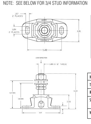
27166 Marine Mounts are compact, captive marine isolators designed to support light to medium loads from 138-750 lbs. per mount.
