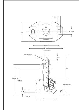
27391 Marine Mounts are compact, captive marine isolators designed to support medium loads from 125-1000 lbs. per mount.
