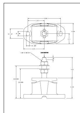
27458 Marine Mounts are compact, captive marine isolators designed to support medium to heavy loads from 350-1,980 lbs. per mount.
